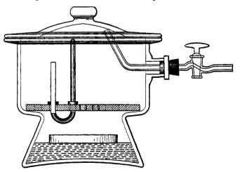
with this mixture. For the ground joint between the desiccator and its cover a vaseline and beeswax mixture is used. The
